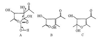
Decarboxylation with concomitant elimination of water could yield B. Cyclization to C followed by loss of water could give the furenidone 13. In support of this hypothesis condensation of pyruvic acid with the dihydroxy diketone 8 does indeed furnish the furenidone 13.
